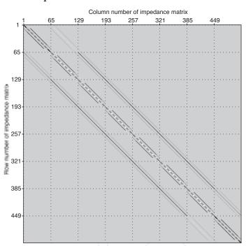
Fig. 2. Pattern of the square impedance matrix discretized with the 27-point mixed-grid stencil (Operto et al.; 2007). The matrix is band diagonal with fringes. The bandwidth is  $O(2N_1N_2)$  where  $N_1$  and  $N_2$  are the two smallest dimensions of the 3D grid. The number of rows/columns in the matrix is  $N_1 \times N_2 \times N_3$ . In the figure,  $N_1 = N_2 = N_3 = 8$
