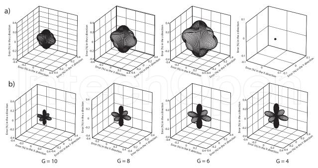
Fig. 3. Phase-velocity dispersion shown in spherical coordinates for four values of G. (a) The phase-velocity dispersion was minimized for G = 4. (b) the phase-velocity dispersion was minimized for 4 values of G: 4, 6, 8 and 10.
