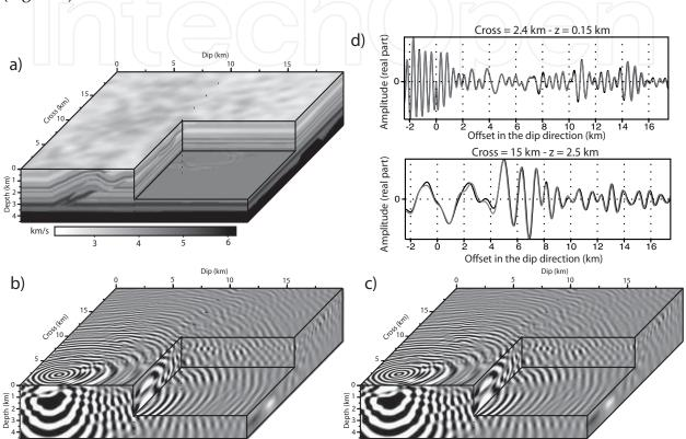
Fig. 7. (a) Overthrust velocity model. (b-c) 7-Hz monochromatic wavefield (real part) computed with the FDFD (b) and FDTD (c) methods.(d) Direct comparison between FDFD (gray) and FDTD (black) solutions. The receiver line in the dip direction is: (top) at 0.15-km depth and at 2.4 km in the cross direction. The amplitudes were corrected for 3D geometrical spreading; (bottom) at 2.5-km depth and at 15 km in the cross direction.
