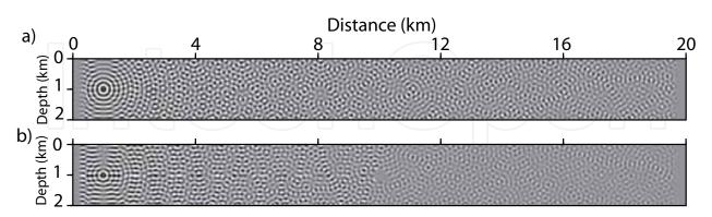
Fig. 11. Pressure wavefield in the oceanic waveguide without (a) and with (b) a circular cavity in the water column. Note that two 500-m layers of PML absorbing conditions are implemented at the two ends of the model.
