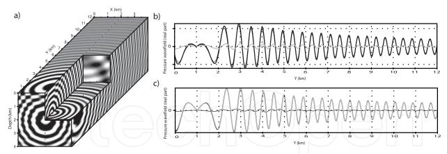
Fig. 5. a) Real part of a 3.75-Hz monochromatic wavefield in a homogeneous half space. (b) Comparison between numerical (black) and analytical (gray) solutions at receiver positions. The Sinc interpolation with 4 coefficients was used for both the source implementation and the extraction of the solution at the receiver positions on a coarse FD grid.
