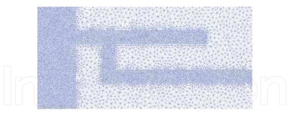
Fig. 14. Zoom on the gallery model mesh. Note the size of cells adapted to local wavespeed.
