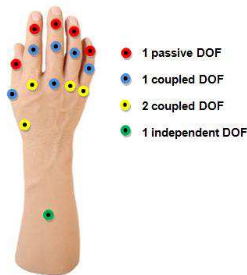
Fig. 7. Kinematic architecture of the proposed prosthesis
