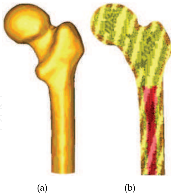
Fig. 10. a) FE model of healthy femur, b) Coronal section of healthy femur model
