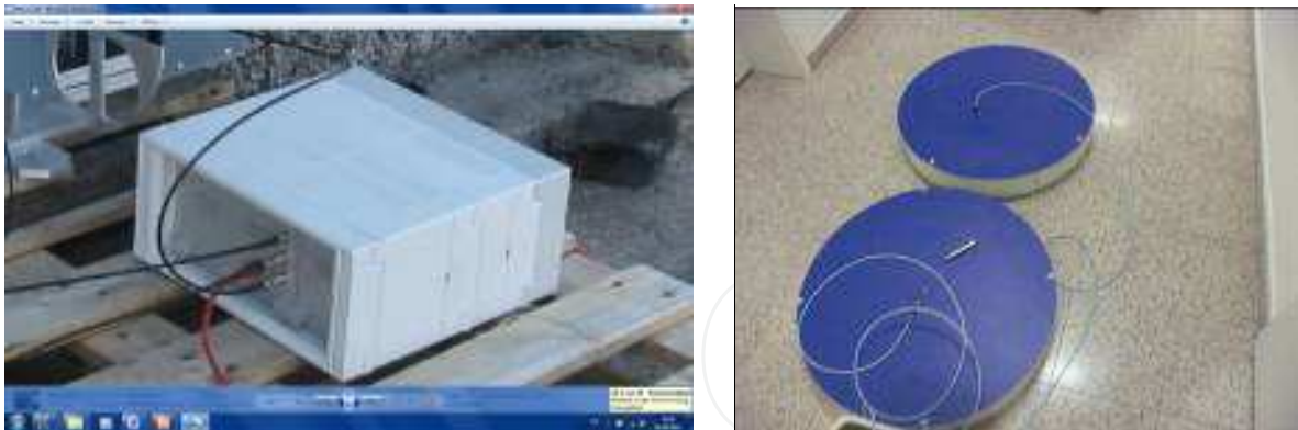
Fig. 2. Radar device and antennas used in prototype system. Courtesy to MEODAT, Ilmenau and IRK, Dresden.
