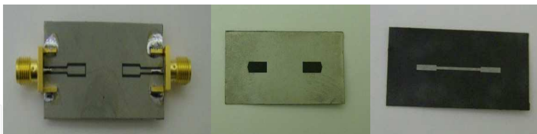
Fig. 6. Photograph of the fabricated UWB filter.
