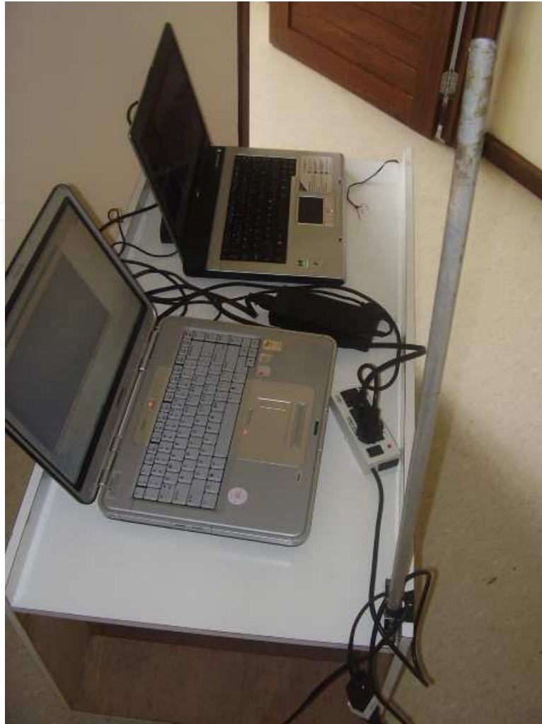
Fig. 6. The cart with notebook running Network NetStumbler (the lower side of the picture) and the notebook running VoIP calls (the upper side of the picture)
