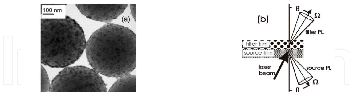
Fig. 21. (a) TEM image of 420 nm PS beads, which are LbL-coated by CdTe NCs in one deposition circle. The NCs appear darker due to the higher contrast. (b) Layout of the PL measurements. \theta - the angle of incidence and the angle of detection, \Omega - the solid angle of the light collection.
