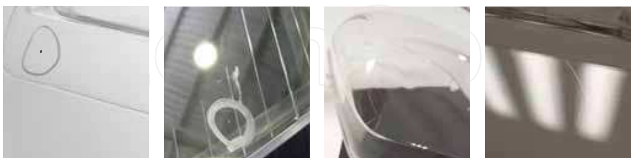
Fig. 2. Aesthetic defects. From left to right: punctual and opaque defect (a black point), punctual and transparent defect (a blister), lineal defect (a scratch) and surface defect (excesses of varnish).
