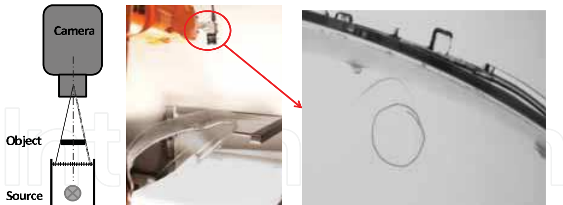
Fig. 9. Diffuse back-light. From left to right: principle of lighting; robotic platform with back-light illumination; the image acquisition.
