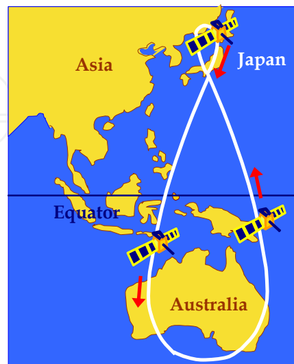
Fig. 42. Apparent orbits of three planned 24-hour QZSS-satellites with inclination i = 45^\circ and eccentricity e = 0.099 .
