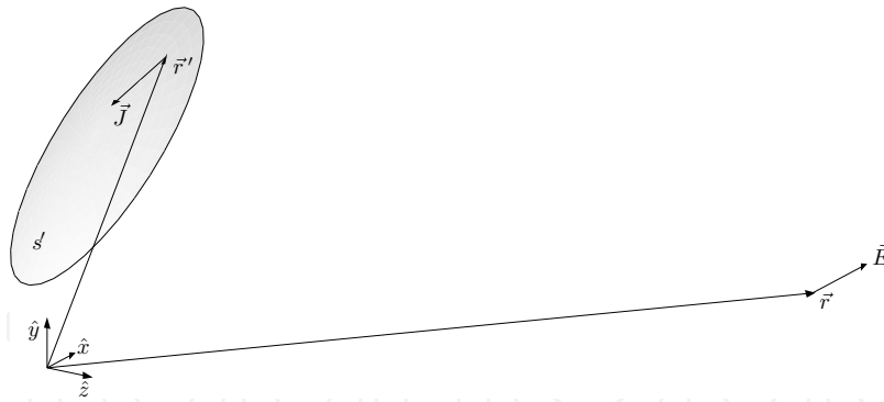
Fig. 9. Farfield \vec{E} at observer point \vec{r} relative to a current distribution \vec{J} at source points \vec{r}' over s' .
