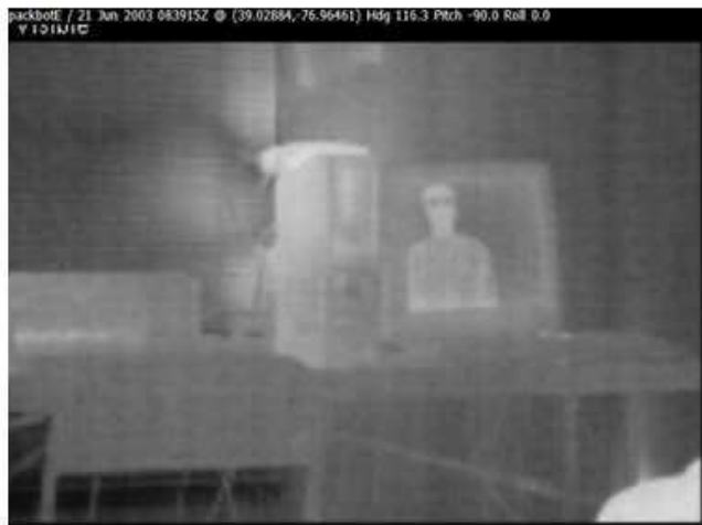
Fig. 20. IR image frame showing thermal reflection of person in front of the computer
