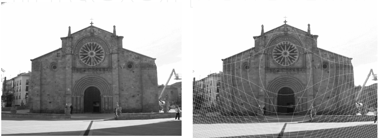
Fig. 5. Left: original image with radial distortion. Right: image without radial distortion, corrected by the direct method.
