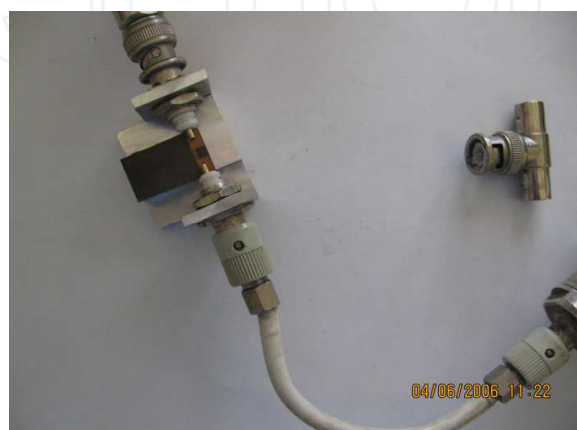
Fig. 7. The active structure of the micromixing device mounted on the test fixture
