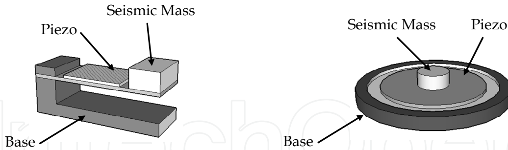
Fig. 2. Cantilever and diaphragm electromechanical structures for energy harvesting.
