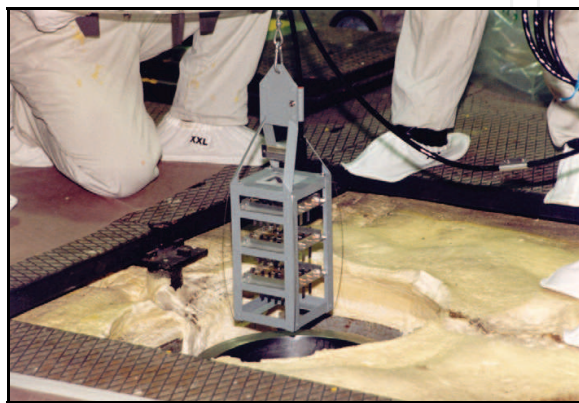
Fig. 12. Insertion of rack with mass-change specimens and electrical resistance sensor into the reactor containment
