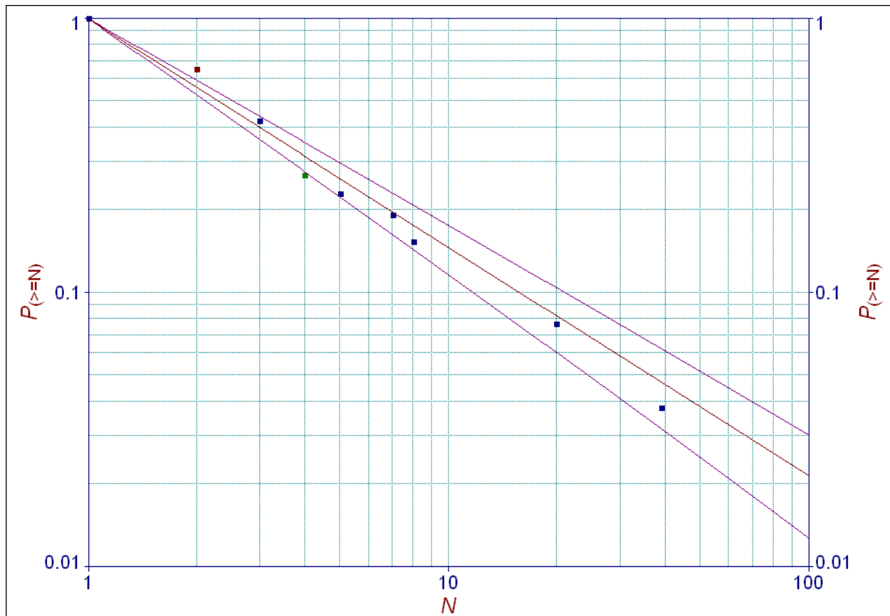
Fig. 9. Cumulative probability of an accident with N or more fatalities as a function of N for all accidents with fatalities, related to storage activity in the downstream oil industry (TNO Database FACTS entries over the time period 1938-2008).
