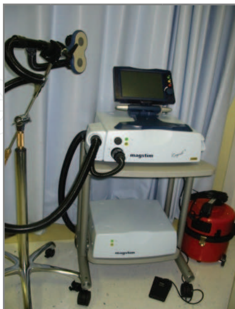
Fig. 4. Magstim super-rapid 2 TMS device at BNL that can deliver pulses reaching up to 100 Hz.
