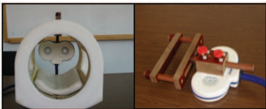
Fig. 7. Picture of the TMS coil holder developed at Brookhaven National Laboratory; left: RF-coil, TMS coil, and coil holder; and, right: TMS coil and coil holder.
