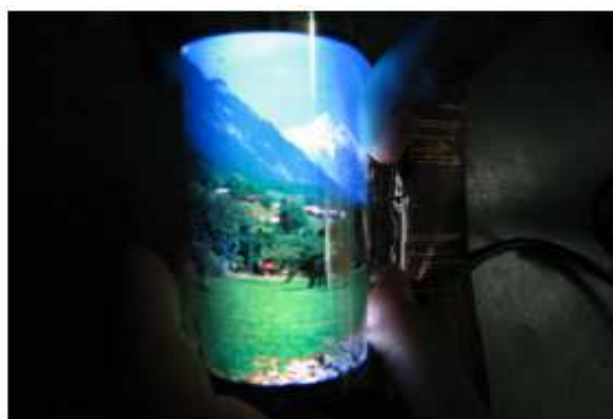
Fig. 28. 6.5" flexible AMOLED display by Samsung. ufigure LOGICAL ISSUES FOR SMALL-SIZED MOBILE OLEDD
