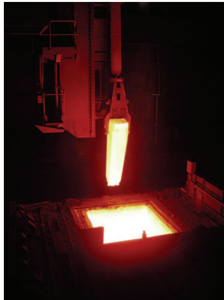
Fig. 1. An ingot for bearing steel production is lifted out of a soaking pit furnace at Ascométal in France. The furnace is fired with flameless oxyfuel, heating the ingots uniformly to over 1200°C.
