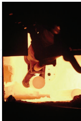
Fig. 13. A look through the furnace door of the rotary hearth furnace at ArcelorMittal Shelby, USA; a flameless oxyfuel burner is firing straight towards the open door. Here the conversion from air-fuel to flameless oxyfuel led to a 60% reduction of the CO 2 emission.
