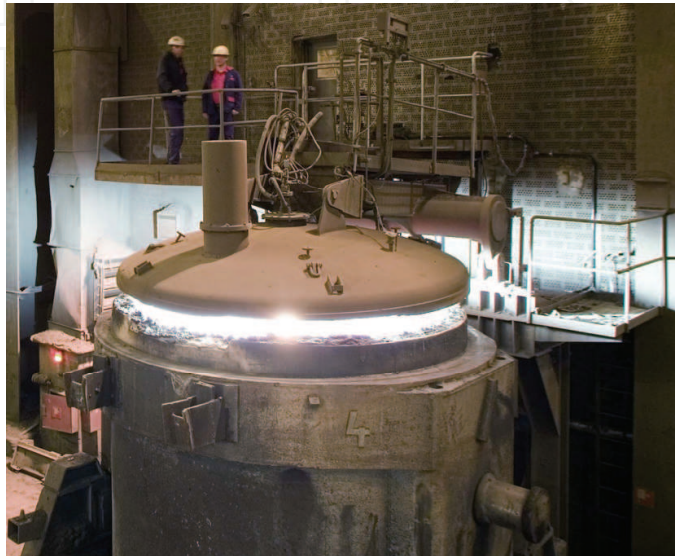
Fig. 7. Ladle preheating using flameless oxyfuel at Ovako's Hofors Works, Sweden.
