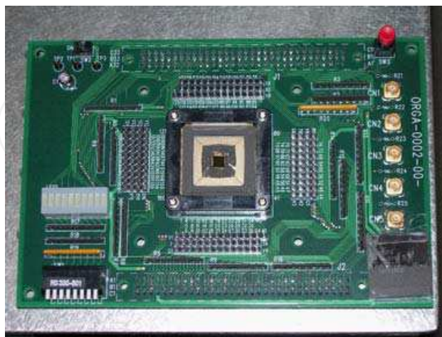
Fig. 6. Photograph of an ORGA-VLSI board with a fabricated ORGA-VLSI chip. The ORGA-VLSI was fabricated using a 0.35\ \mu\text{m} three-metal 4.9 \times 4.9\ \text{mm}^2 CMOS process chip. The gate count of a gate array on the chip is 68. In all, 340 photodiodes are used for optical configurations.
