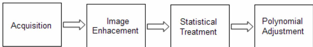
Fig. 4. Flow diagram of the algorithm for image processing
