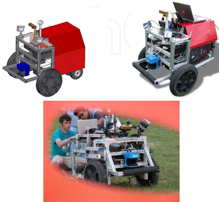
Fig. 8. Bearcat Cub intelligent vehicle designed for IGVC
