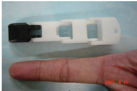
Fig. 7. Finger profile comparisons for a twenties volunteer and the proposed robot hand
