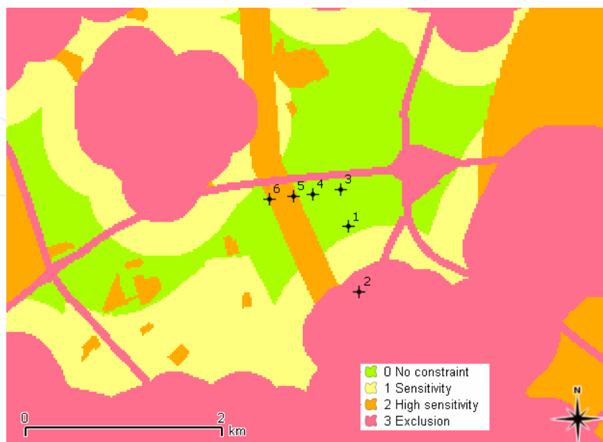
Fig. 10. Overlay of the location of a wind farm project and the composite constraints map.
