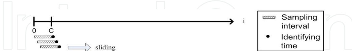
Fig. 4. Periodical interval checking for identifying LOS/NLOS status
