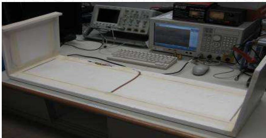
Fig. 3. Prototype of RFID reader antenna
