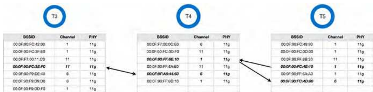
Fig. 4. An example of a chain of border APs and a list of preferred APs in T3, T4 and T5 stations
