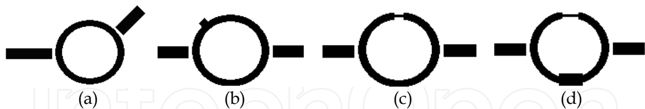
Fig. 4. Dual mode microstrip line ring resonators: (a) unequal length arms, (b) patch in one arm, (c) notch in one arm, and (d) different characteristic impedances of the arms.
