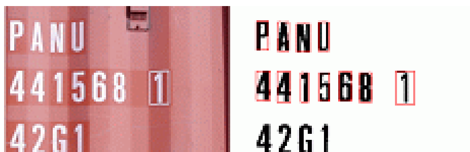
Fig. 5. Identifier area with a general color and successful results of edge extraction
