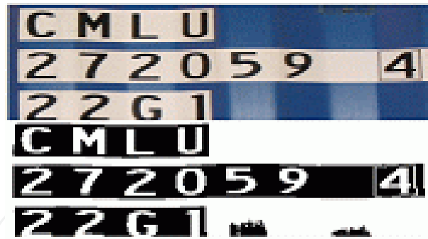
Fig. 6. Identifier area with white color and failed results of edge extraction
