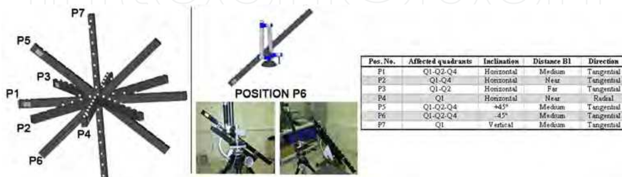
Fig. 2. Ball bar positions for each quadrant. Sample of position P6.
