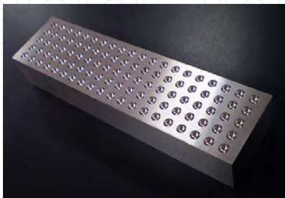
Fig. 1. Example of a target LED lens mold. Each diameter of concaved area is 4 mm.
