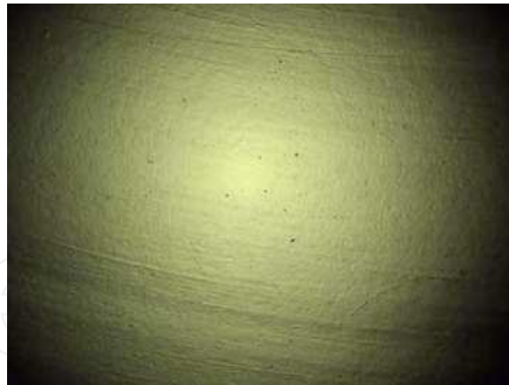
Fig. 14. Large scale photo of the LED lens mold after the finishing process by partially using the proposed stick-slip motion control.
