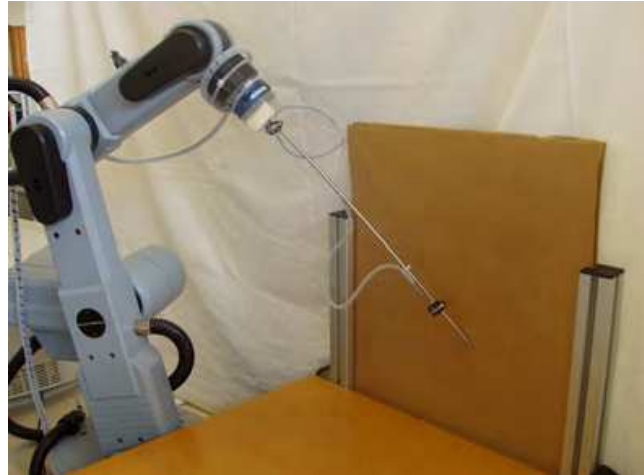
Fig. 2. Steel rod impact against a rigid surface
