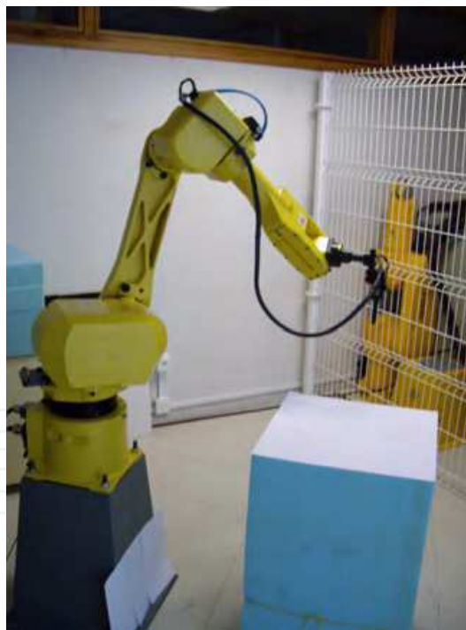
Fig. 9. The FANUC Arc Mate 100iB. The parallelepiped foam obstacle is shown in the bottom right corner.
