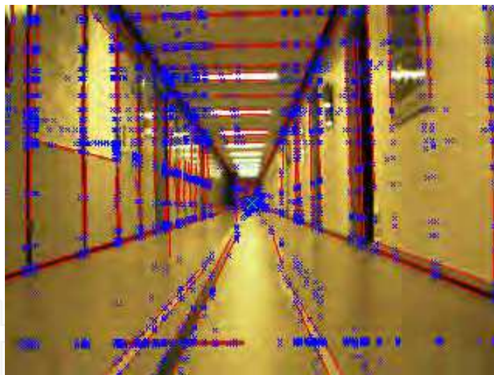
Fig. 7. The illustration of the vanishing point extraction. The extracted lines are shown in red, the vanishing point candidates are shown in blue and the green cross at the center is the detected vanishing point.
