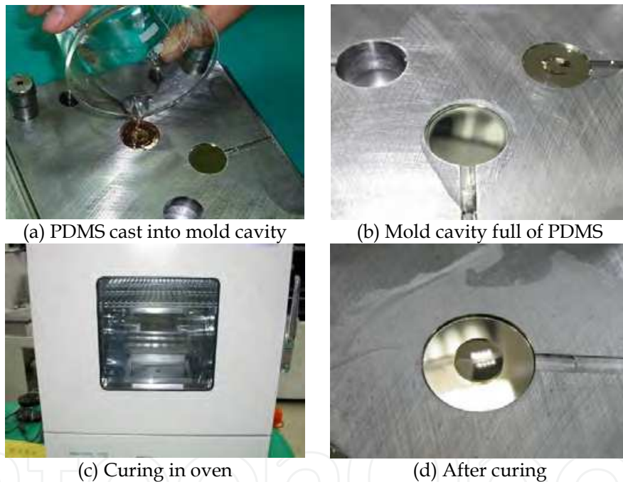
Fig. 5. Fabrication processes of PDMS lens.
