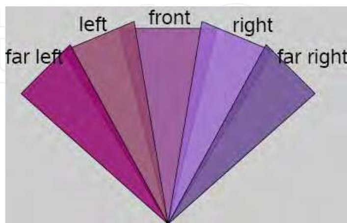
Fig. 3. A symmetric arrangement of five directional distance sensors for visual steering.
