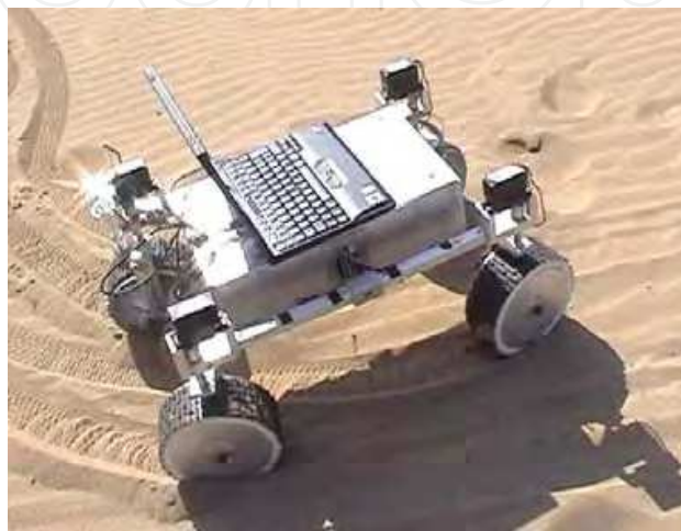
Fig. 1. Significant wheel slip and sinkage of the rover Dune, constructed at the University of Salento
