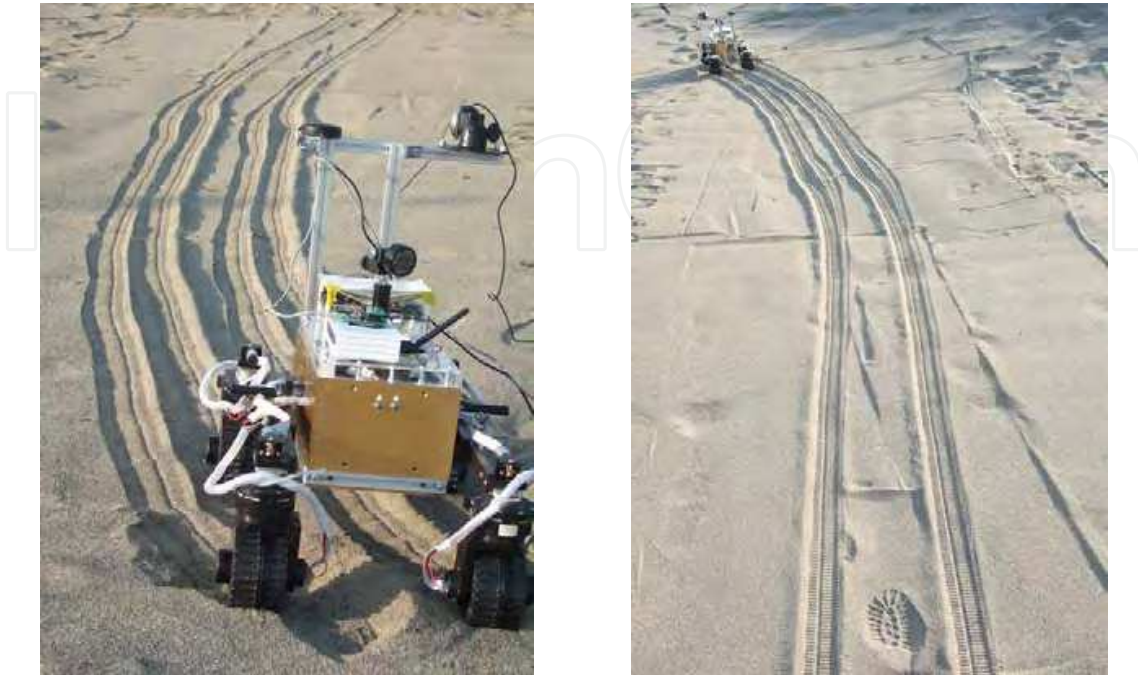
Fig. 11. Position of the rover and wheel traces at the end of the traverse of a sandy slope: a) Front view, b) rear view
