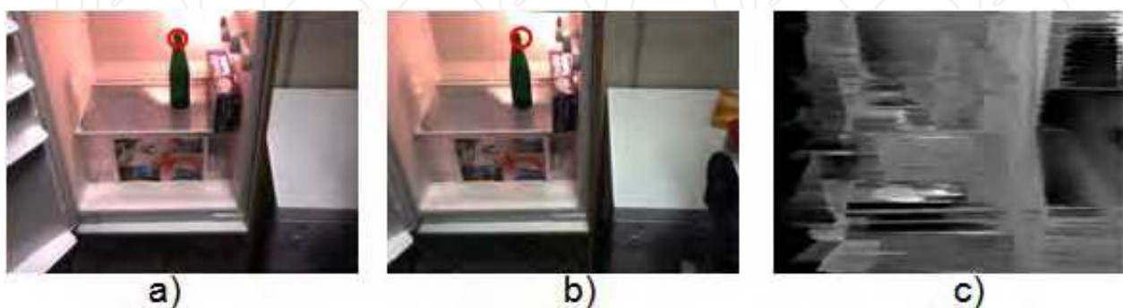
Fig. 11. Disparity map for bottle position 2; stereo images a) Left b) Right; c) Disparity map
