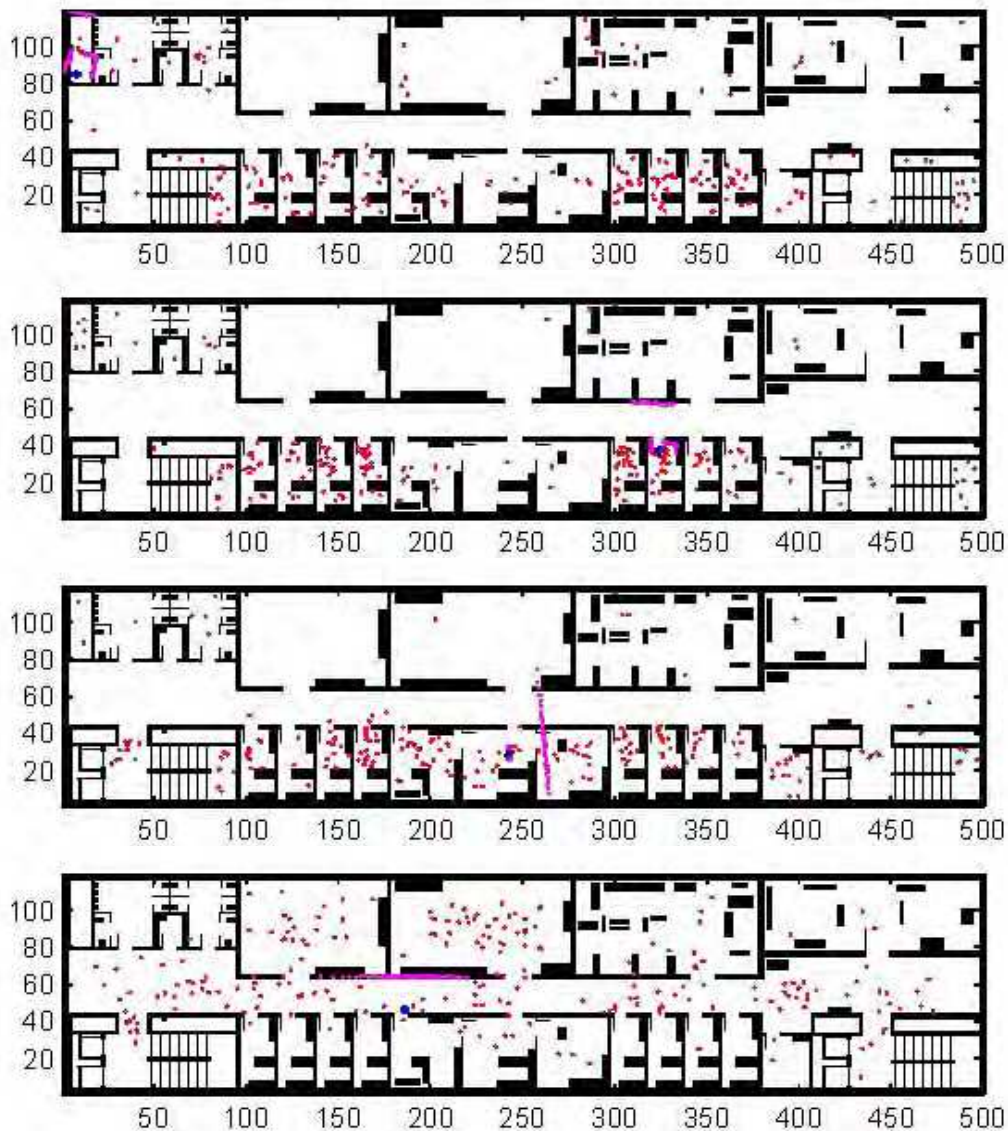
Fig. 4. Convergence failure, starting pose (305, 30, 270), 200 elements in population and \sigma of 1% of the measured signal, motion +2.5 cells per cycle in y direction.
