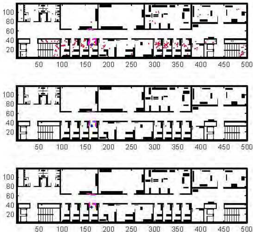
Fig. 3. Premature hypothesis elimination, starting pose (305, 30, 270), 200 elements in population and \sigma of 3% of the measured signal, motion +2.5 cells per cycle in y direction.
