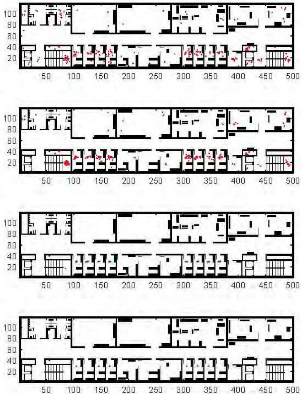
Fig. 2. Premature hypothesis elimination, initial pose (105, 30, 270), 200 elements in population and \sigma of 3% of the measured signal.
