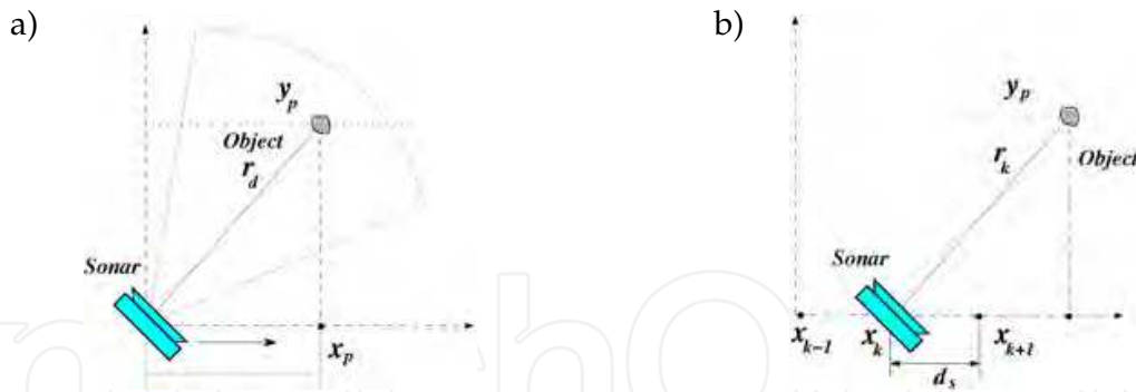
Fig. 15. a) A robot equipped with an ultrasonic sonar moves along a straight line and passes by an object. b) The measurements of the distance to an object are performed at the points regular spread along the robot path
