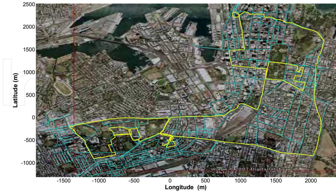
Fig. 8. Estimated path (in yellow) for one of the experiments. The known map (cyan) and a satellite image of the region are included in the picture.
