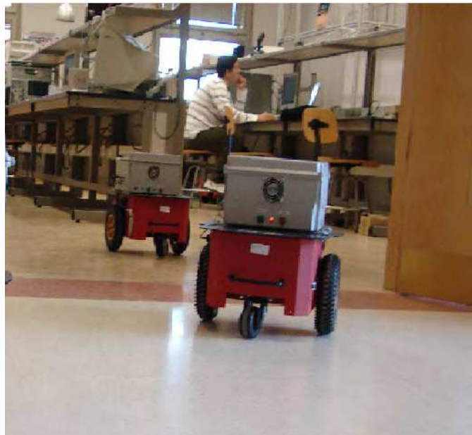
Fig. 12. View of the laboratory set-up of telerobotics applications with P3-DX units.
