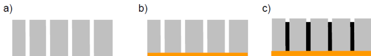
Fig. 7. Schematic of the electrochemical deposition template method: a) nanoporous membrane, b) deposition of a conductive layer on one side of the template, c) growth of the nanowires inside the pores.
