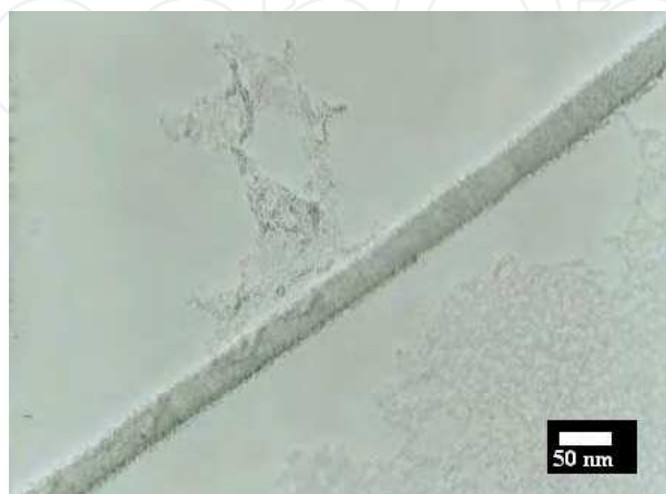
Fig. 3. TEM image of the GaNWs revealing a uniform diameter of \sim 40 nm.
