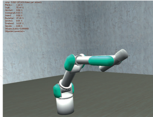
Fig. 22. Animation of the PA10 robot in Blender
