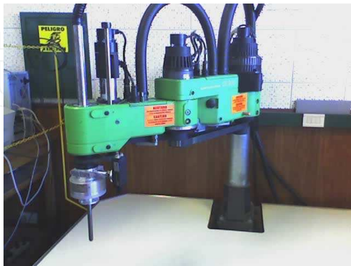
Fig. 9. Industrial robot manipulator Bosch SR-800, at the National University of San Juan, Argentina
