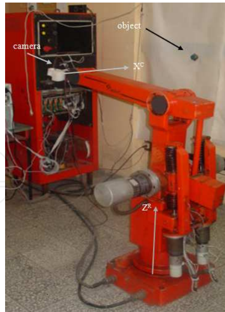
Fig. 11. 2D Vision-based control, experimental set-up
