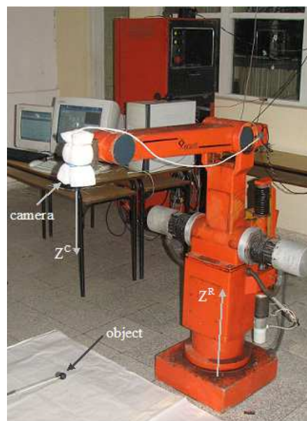
Fig. 14. 3D Vision-based control, experimental set-up
