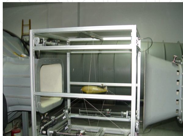
Fig. 7. Second WDPSS prototype in open return circuit LSWT for blowing test
