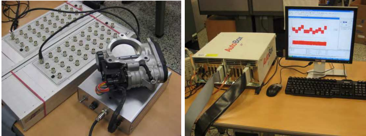
Fig. 13. Photograph of workstation with modular dSPACE hardware in Autobox
