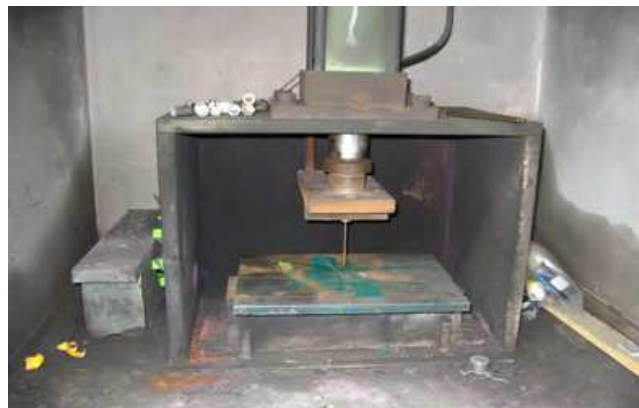
Fig. 1. Nail penetration Test equipment.
